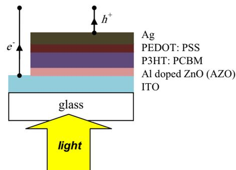
Fig. 1. Schematic structure of inverted type of organic solar cells based on P3HT:PCBM with AZO as its electron transport layer.
