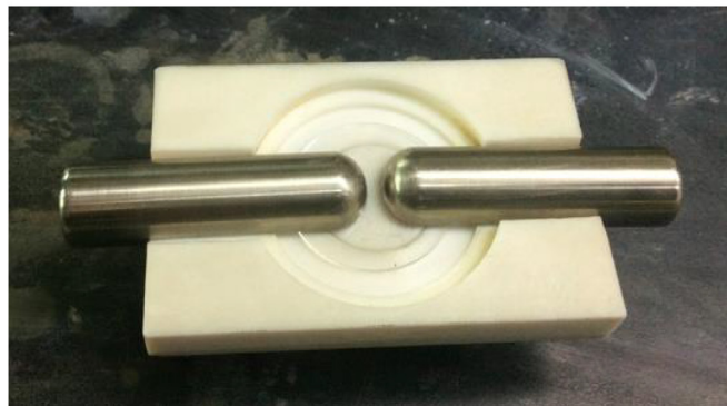
Fig. 1. (a) The schematic of nanosecond pulse flashover testing platform. The nanosecond pulse is generated by a MARX pulse generator. And the flashover testing is performed in a vacuum chamber. (b) The sample holder for flashover testing.
