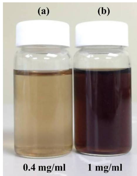
Fig. 1. Digital pictures of graphene oxide suspensions with concentration of 0.4 mg/ml (a) and 1 mg/ml (b) created by GO powders dispersed in 100 ml of deionized water.
