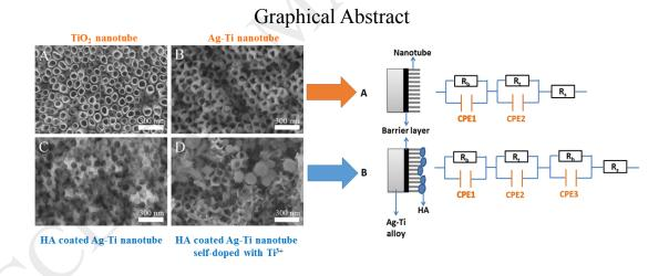
Ag-Ti nanotube array was prepared and uniform hydroxyapatite (HA) was electrochemically deposited on the nanotubes. It's found that the Ti<sup>3+</sup> can promote the grow rate of hydroxyapatite coating on nanotube surface and the hydroxyapatite coated nanotube with Ti<sup>3+</sup> exhibit excellent stability and higher corrosion resistance.
