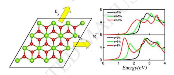
The in-plane stiffness of  $PtX_2$  monolayer are smaller than that of  $MoX_2$  monolayers. Moreover, the tensile strain can affect obviously the electronci structures and optical properties of  $PtX_2$  monolayer.
