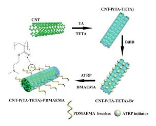
A novel and effective approach for non-covalent functionalization of carbon nanotube via the mussel inspired polymerization of tannic acid and triethylenetetramine and subsequent surface initiated atom transfer radical polymerization method.
