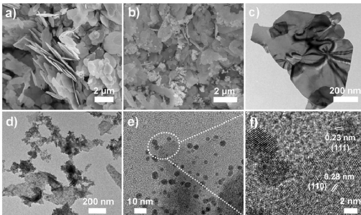
Fig. 1. SEM (a and b), TEM (c, d, and e), and HRTEM (f) images of BiOI (a and c) and Pt–BiOI (b, d, e, and f) samples.
