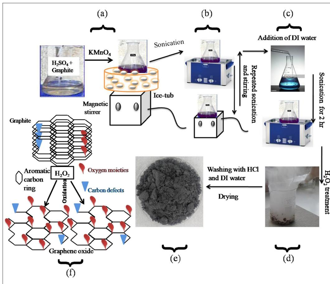
**Fig. 1.** (a–d) show the addition of constituents chemicals (i.e., graphite powders,  $\text{H}_2\text{SO}_4$  and  $\text{KMnO}_4$ ), ice-bath, magnetic stirring, sonication, quenching of reaction via addition of DI water and oxidation steps in the synthesis of GO. (e) Shows the dried GO powder. (f) Shows the schematic of carbon defects, broken bonds in the aromatic ring and attachment of functional oxygen groups in the GO sheets.
