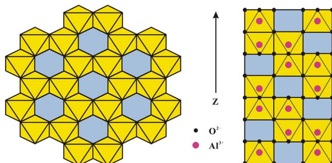
Fig. 2. α-Al<sub>2</sub>O<sub>3</sub> super cell model. Polyhedra have been drawn to show the coordination of each cation.
