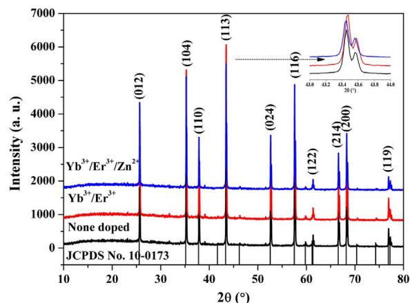
Fig. 1. XRD patterns of none doped, Er<sup>3+</sup>/Yb<sup>3+</sup> and Er<sup>3+</sup>/Yb<sup>3+</sup>/Zn<sup>2+</sup> doped Al<sub>2</sub>O<sub>3</sub> transparent ceramics (in set is enlarged XRD patterns of (113)).
