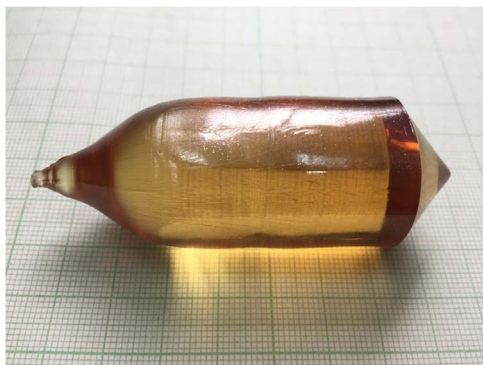
Fig. 1. Photo of the as-grown Pr:YAP crystal.
