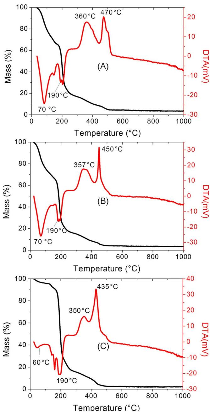
Fig. 1. TGA/DTA analysis performed for precursors obtained from solutions of (A)  $\text{Sr}^{2+}$  and  $\text{Ce}^{3+}$  (B)  $\text{Sr}^{2+}$ ,  $\text{Ce}^{3+}$  and  $\text{Ag}^+$  and (C)  $\text{Sr}^{2+}$ ,  $\text{Ce}^{3+}$ ,  $\text{Ag}^+$  and  $\text{Eu}^{3+}$ .
