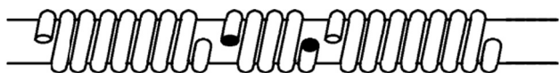
Fig. 1. Sketch of 4-turn rf coil with 8-turn coil extensions along the sample tube. The coil lead wires are represented as filled circles, with the leads oriented in/out of the page. The extensions' wires start and stop at the extensions (no leads). In use, the extensions are moved axially to be in contact with the rf coil. All segments are close-wound, in practice.
