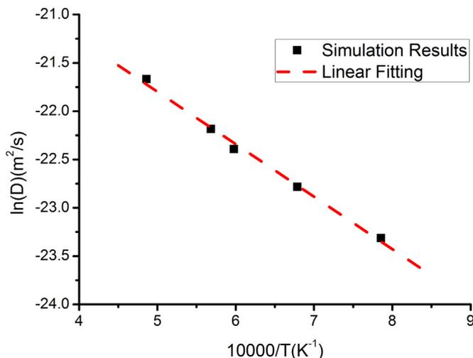
Fig. 2. Arrhenius plot showing the diffusion coefficient ( $D$ ) of oxygen ions as a function of  $1/T$  for 8 mol%  $Y_2O_3$  concentrations in cubic yttria-stabilized zirconia.
