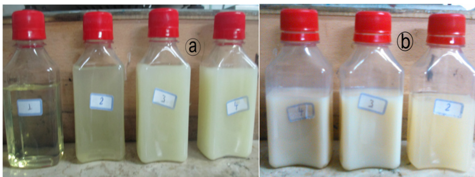
Fig. 1. Dispersion of nanoparticles (a) TiO 2 + engine oil (b) TiO 2 + engine oil + surfactant.
