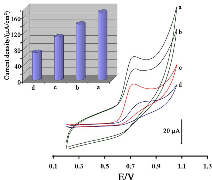
**Fig. 3.** Cyclic voltammograms of 500.0  $\mu\text{M}$  raloxifene at a surface of a) CPE/NiO/SWCNTs/1B4MPTFB; b) CPE/1B4MPTFB; c) CPE/NiO/SWCNTs and d) CPE at pH = 7.0. Inset) current density obtained from this figure's data. Condition; Scan rate 100 mV/s and pH = 7.0.
