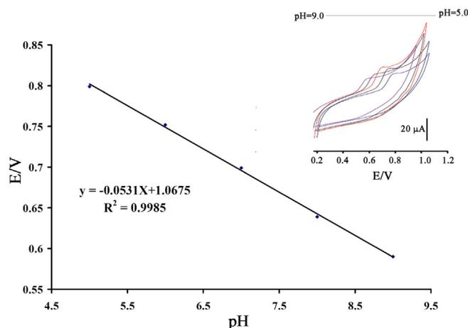
**Fig. 2.** Potential-pH curve for electro-oxidation of 300.0  $\mu\text{M}$  raloxifene at a surface of CPE/NiO/SWCNTs/1B4MPTFB in the pH range 5.0–9.0. Inset) relative cyclic voltammograms of 300  $\mu\text{M}$  raloxifene at a surface of CPE/NiO/SWCNTs/1B4MPTFB in the pH range 5.0–9.0.
