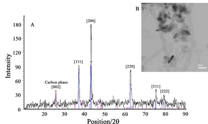
**Fig. 1.** A) XRD pattern of NiO/SWCNTs nanocomposite. B) TEM image of NiO/SWCNTs nanocomposite.
