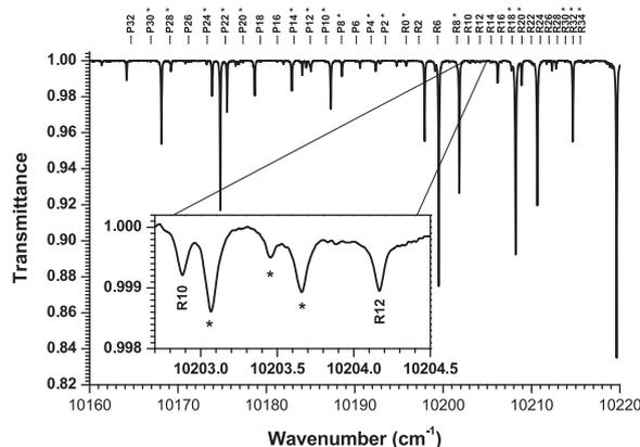
Fig. 2. Fourier transform spectrum of the carbon dioxide sample in the 10160–10220 cm<sup>-1</sup> region ( $P=294$  mbar,  $L=953.6$  m,  $T=294$  K). All strong lines belong to the water vapor. The insert shows R10 and R12 lines of the 60014-00001 band of <sup>12</sup>C<sup>16</sup>O<sub>2</sub>. The water lines in the insert are marked with the asterisks.
