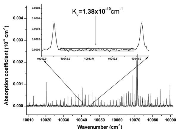
Fig. 1. Survey spectrum of CO<sub>2</sub> in the 10010–10090 cm<sup>-1</sup> region:  $P=294$  mbar,  $L=953.6$  m,  $T=294$  K. The insert demonstrates the sensitivity of the setup.
