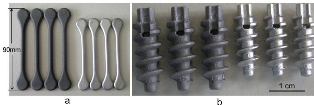
Fig. 2. a: dogbone shape tensile test specimen [12] in: green condition (after injection moulding of the plasticised feedstock granules)- sintered condition (right side). b: suture anchor implant screw demonstrator parts made by MIM of EZK400 powder material in the green and sintered condition. Design: ConMed, USA.
