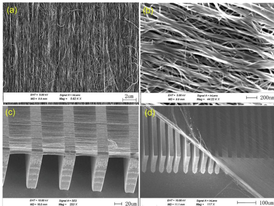
Fig. 1. SEM representation: (a) and (b) SEM photos of CNT sheet; (c) and (d) SEM photos of CNT@Grating. (A colour version of this figure can be viewed online.)
