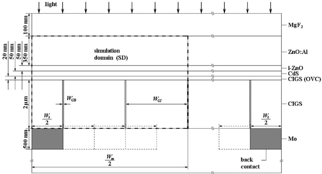
**Fig. 1.** Modeled and simulated CIGS solar cells with localized back contact. The width of the finger and module is denoted with  $W_f$  and  $W_m$ , respectively. The structure with a whole back contact is obtained when  $W_f$  equals  $W_m$ . The vertical grain boundaries (GBs) inside the CIGS are also modeled: the widths of the GB and the grain are denoted by  $W_{GB}$  and  $W_{GI}$  ( $W_{GB}=25 \text{ nm}$ ,  $W_{GI}=2 \mu\text{m}$ ).
