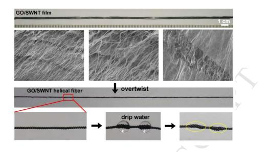
A continuous single-walled carbon nanotube (SWNT) network into dispersed GO sheets to fabricate GO/SWNT composite films and helical fibers with an alternating layered structure which lead to reversible mechanical actuation with axial contraction up to 50% of original fiber length in response to water adsorption.
