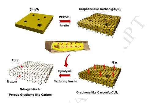
A protocol for  $g-C_3N_4$  template-directed fabricating nitrogen-rich porous graphene-like carbon sheets (NPGCs) has been developed by using plasma-enhanced chemical vapor deposition followed with high-temperature pyrolysis. As supercapacitor electrode, the NPGCs deliver quite encouraging specific capacitance, high rate capability and outstanding cycle performance.
