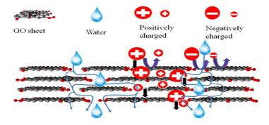
The schematic view for water pass though route and the rejection mechanism for charged organic dyes.
