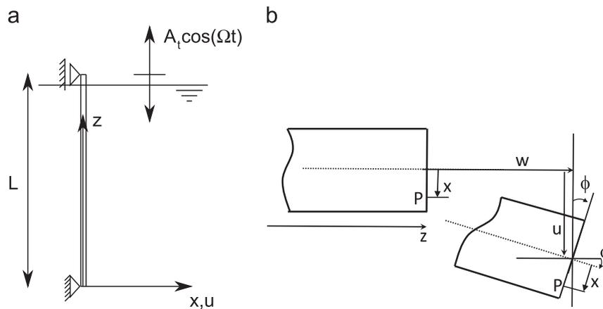
**Fig. 1.** Schematic representations of the flexible rod: (a) Sketch of the vertical rod and (b) Bernoulli–Euler beam model.  $\phi$  is the angle between the beam axis in the original and deformed configurations.
