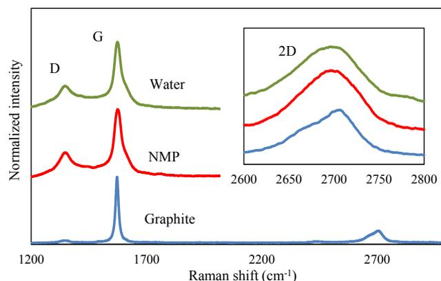
Fig. 1. Raman spectra of graphite powder and of thin film prepared after 1 h sonication for NMP and water based dispersion. Inset: Detailed 2D Raman bands. (A colour version of this figure can be viewed online.)
