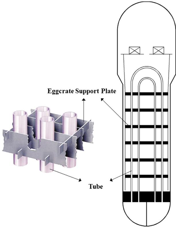
Fig. 1. Schematic of the stream generator and eggcrate support plate.
