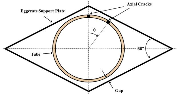
Fig. 2. Schematic of crack locations in the tube.
