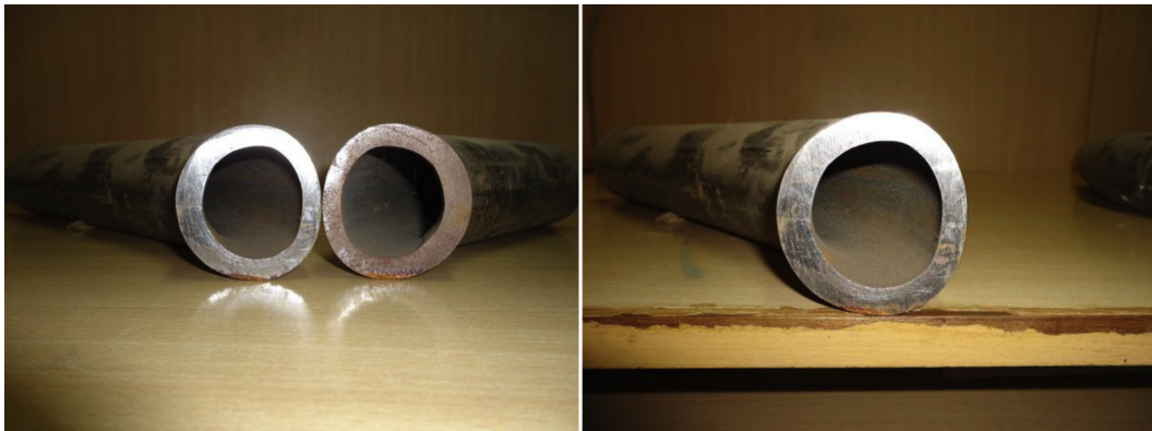
Fig. 1. Actual cold bent pipes with deviation in cross section and wall thickness (Courtesy, GB Engineering, Tiruchirappalli.).
