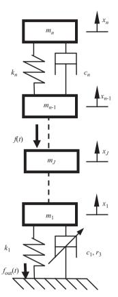
Fig. 1. MDOF structure on a support base with a cubic non-linear damping.
