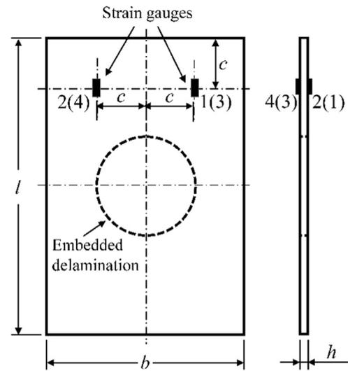
Fig. 1. Geometry of a specimen with circular delamination.
