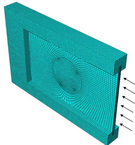
Fig. 3. Finite element model.
