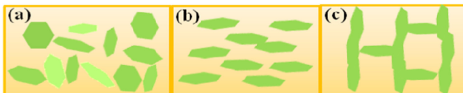
Fig. 1. Schematic description of GNP dispersion in polymer matrix: (a) random dispersion, (b) oriented layer-structure and (c) ordered 3D network.
