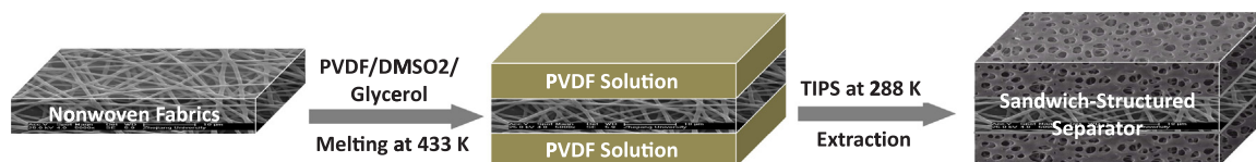
Scheme 1. Schematic representation of the preparation process of SSCS.
