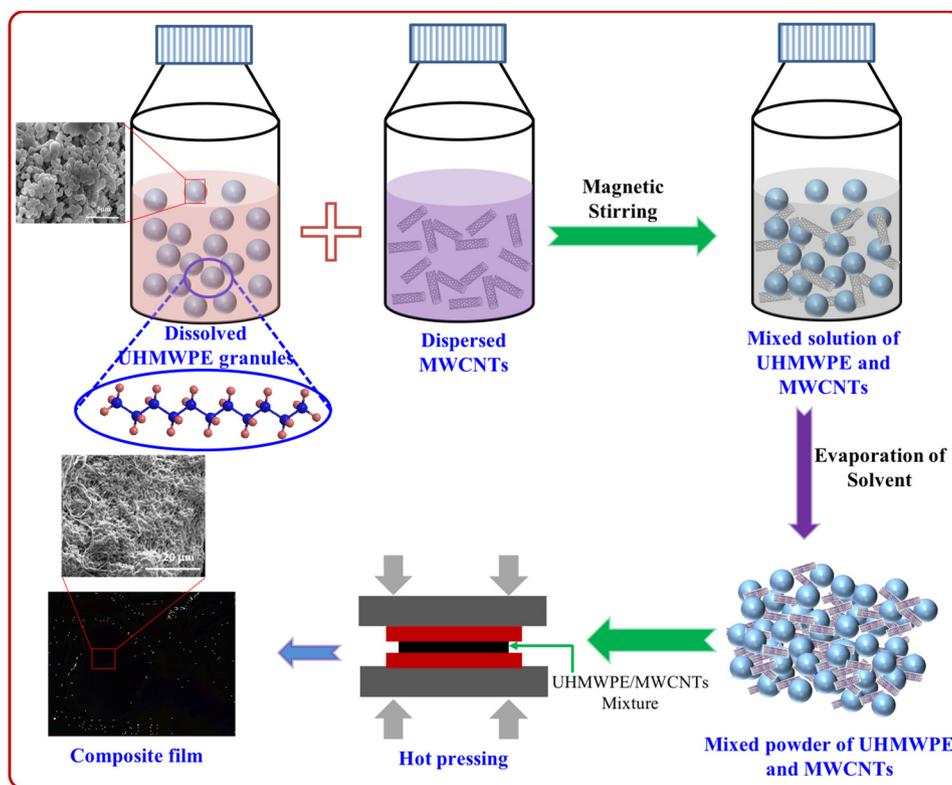
Fig. 1. Schematic of the CNT/UHMWPE fabrication process.
