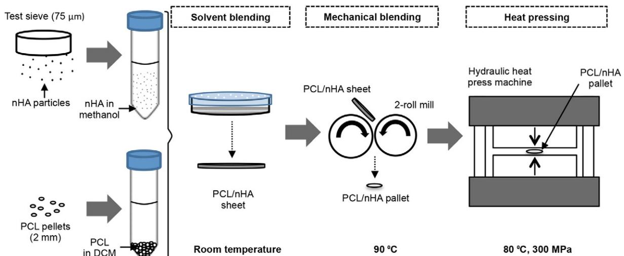
Fig. 1. Schematic diagram illustrating the fabrication processes of PCL/nHA composite film.
