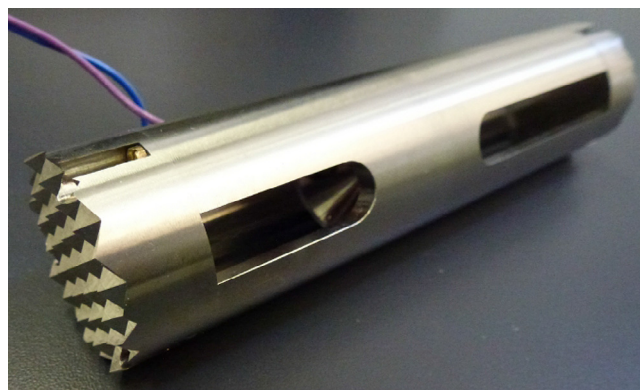
Fig. 1 – Sensor used for speed of sound measurements in compressed liquids. Different path lengths are revealed by the asymmetry of the loops. Pyramids, on the outer surfaces of the reflectors, prevent the transmitted signal to return to the receiver, interfering with the main signal.
