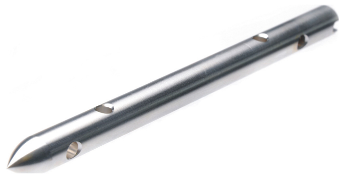
Fig. 1. Intramedullary nail made of magnesium-based alloy LAE442. This test implant had a length of 130 mm and two holes for intramedullary screw fixation at the proximal and distal ends.
