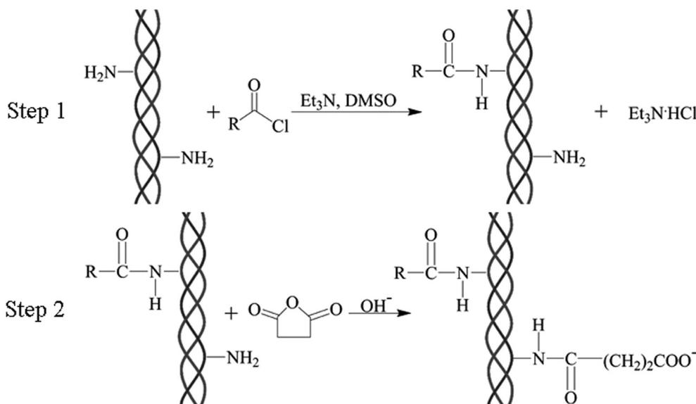
**Scheme 1.** The schematic illustration of acylation of native collagen with lauroyl chloride and succinic anhydride. R:  $\text{CH}_3(\text{CH}_2)_9\text{CH}_2$  – [9].
