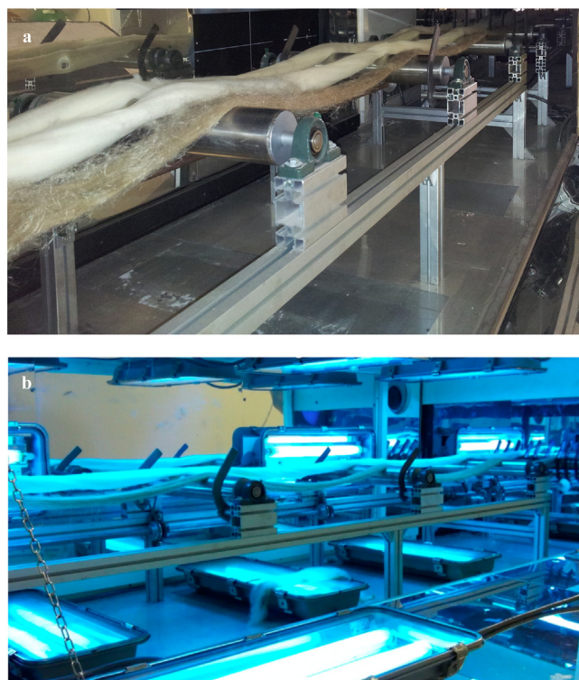
Fig. 1. Pictures of the prototype apparatus developed for the silver deposition treatment of textile substrates. a.) Textile substrates moving toward UV station; b.) UV exposure of the textile substrates.
