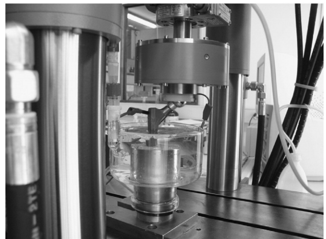
Fig. 2. Mechanical–electrochemical cell used for corrosion–fatigue tests.
