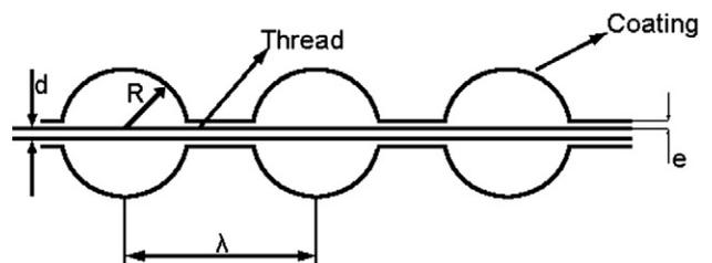
Fig. 2. Typical representation of the beads on a string (BOAS) morphology for the droplets of adhesive on a thread.
