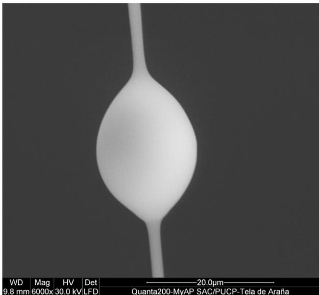
Fig. 1. SEM micrograph of viscid silk showing the typical beads-on-a-string (BOAS) morphology of the adhesive droplets on the silk fibres.
