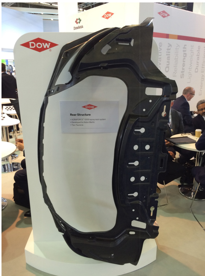
FIGURE 2 Rear structure of an Aston Martin manufactured by Faurecia in VORAFORCE 5300 epoxy resin in a RTM process.
