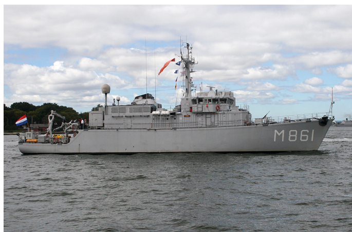
FIGURE 3 The Alkmaar-class MCMV's, like this Zr. Ms. Urk, developed from 1974, has been in service in the Dutch navy since 1983. Its 52 m long, glass fiber reinforced polyester hull was quite revolutionary at the time. Which concept is going to replace it?
