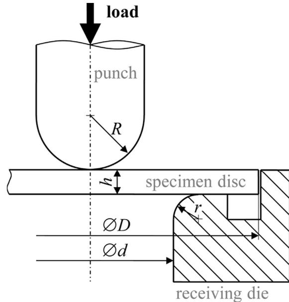
Fig. 1. Sketch of the small punch bending test.
