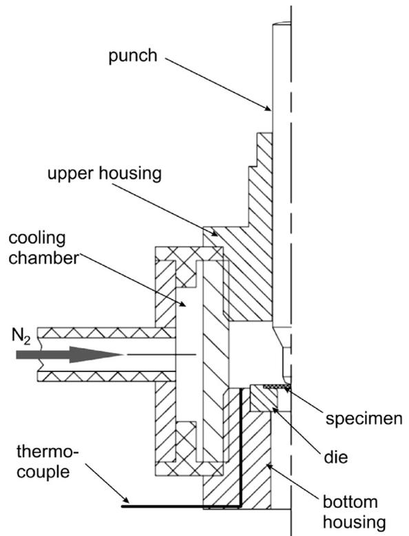
Fig. 2. Half section through cooling chamber (without isolation).
