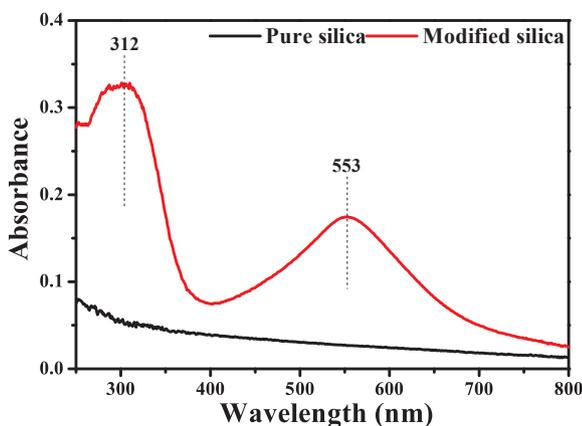
Fig. 3. The UV-vis spectra of pure silica and modified silica coatings.
