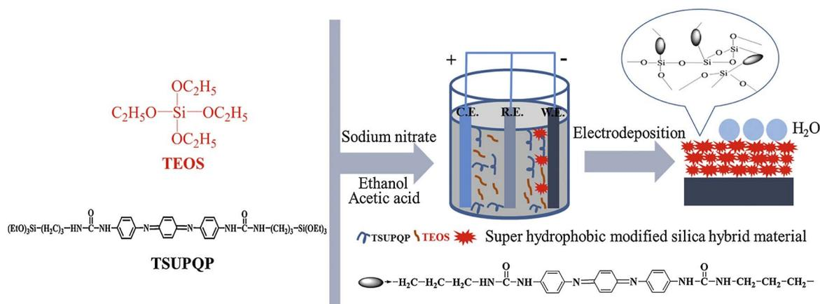
Fig. 1. The schematic diagram of modified silica coating.
