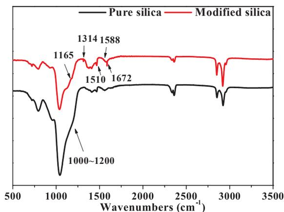
Fig. 2. The FTIR spectra of pure silica and modified silica coatings.
