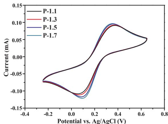
Fig. 4. The CV curves of these hybrid coatings in 0.1 M  $\text{H}_2\text{SO}_4$  solution with the scan rate of 10 mV/s.
