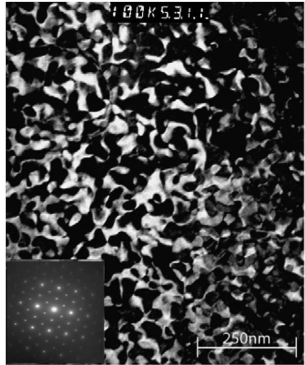
Fig. 1. Dark-field transmission electron microscope image of the structure of Fe–26Al in annealed at 300 °C state: DO<sub>3</sub> domains (in white) immersed into B2 matrix (in black). Reprinted from Ref. [10], copyright 2018, with permission from Elsevier.
