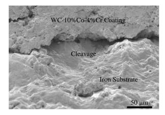
Cleavage cracking of pure iron substrate induced by the fracture of
