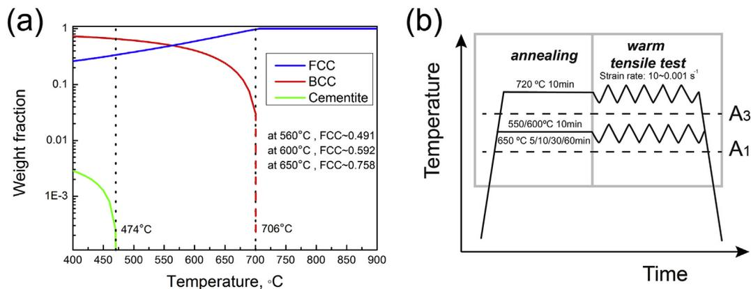
Fig. 1. (a) The equilibrium phase fractions of the alloys at different temperatures, computed using Thermo-Calc with the TCFE9 database, and (b) the schematic diagram showing the thermo-mechanical treatments for warm deformation.
