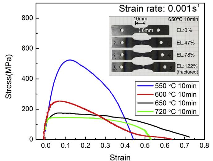
Fig. 2. The stress-strain curves of warm deformation at initial strain rate of 10<sup>-3</sup> s<sup>-1</sup> after pre-annealing for 10 min.
