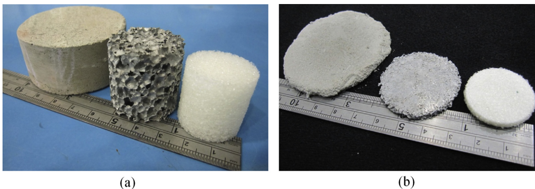
Fig. 1. Photographs of the cement (left), aluminium (middle) and polymer (right) foams: (a) before compression and (b) after densification.
