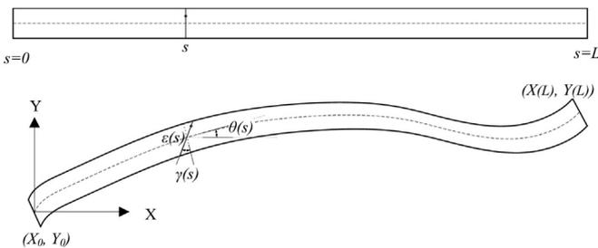
Fig. 1. Description of the configuration of a planar beam with large deformation using its slope angle  $\theta(s)$ , stretch strain  $\epsilon(s)$ , and shear angle or strain  $\gamma(s)$ .
