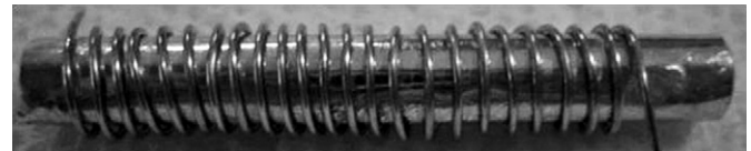
Fig. 2. Coil encircling an X80 steel laboratory specimen.
