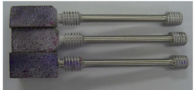
Fig. 2. One set of machined tensile samples, including a sector (left) of the original tube.
