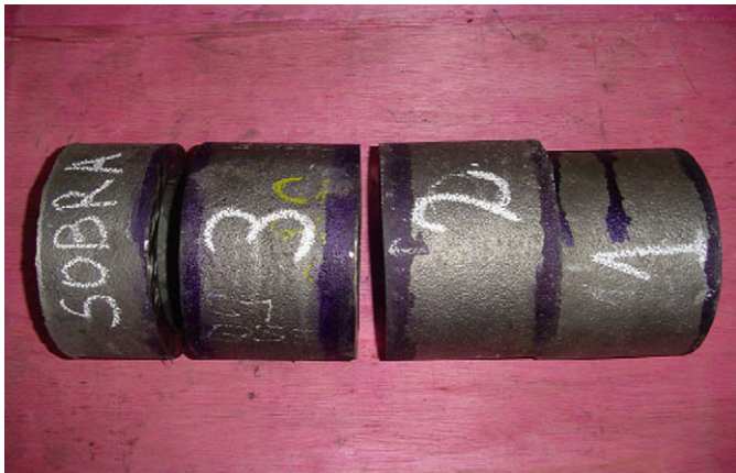
Fig. 1. The centrifugally cast tube investigated in the present work. The tube was cut into four rings (ring number 1 is located in the cold end of the centrifugal casting mold). Rings 1–3 were reserved for the investigation. The last ring (marked as “Sobra” in the picture) was excluded from the investigation.
