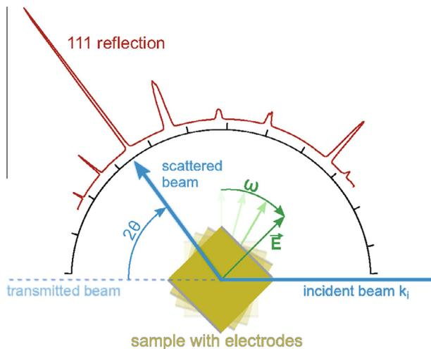
Fig. 1. Experimental setup for analysing all strain mechanisms in one diffraction experiment.
